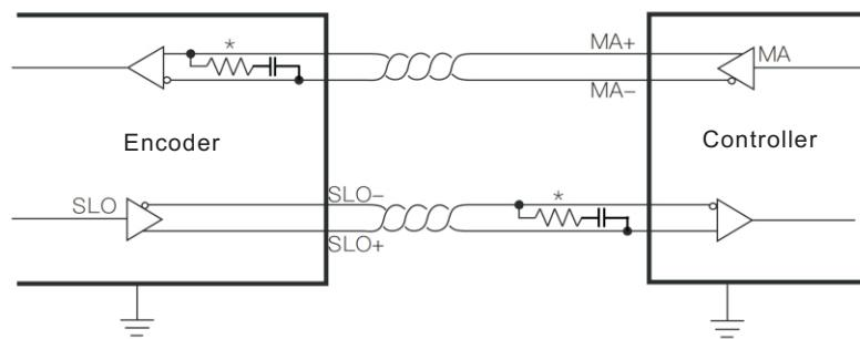
It is a four-wire interface, include the differential lines of MA and SLO. And the terminal resistors of the MA lines have been integrated into the encoder. The users only need to configure terminal resistors or choose other impedance matching schemes for SLO lines.
