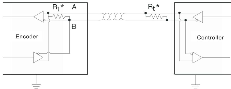
The interface is a two-wire system, which is mainly differential A and B phases. The terminals of the two lines need to be connected to terminal resistors in parallel. The terminal resistors at the encoder end have been integrated into the encoder. Users need to connect terminal resistors or other impedance matching solutions on the controller side A and B.
