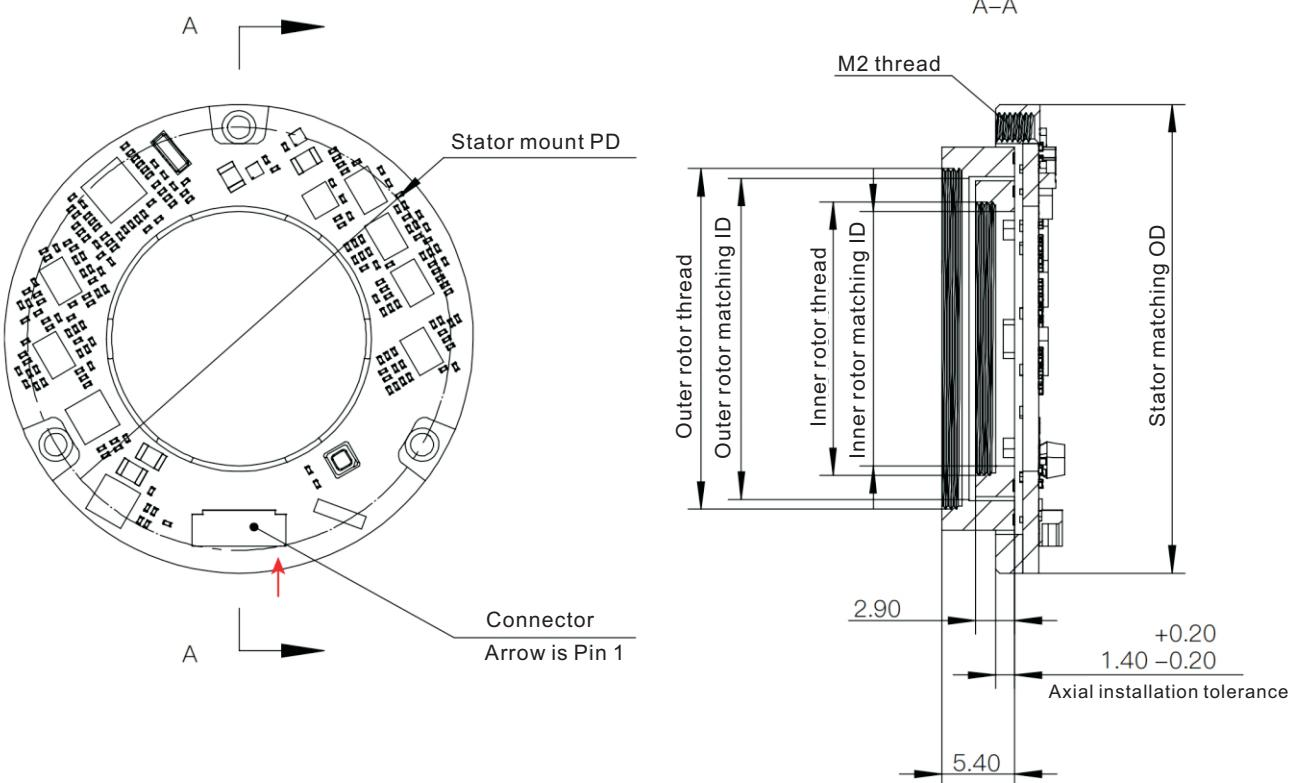
When installing the stator, can use an M1.6 screw to pass through the M2 threaded hole, or can use an M2 thread with an M2 screw to lock it. When installing the rotor, use a special tool to tighten it.
