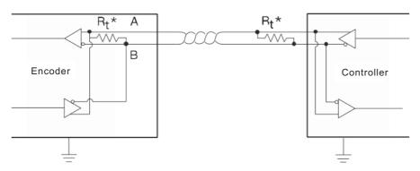
It is a differential two-wire interface, both wires need to be terminated with parallel termination resistors. The terminal resistors have been integrated into the encoder. The users only need to configure terminal resistors or choose other impedance matching schemes for the differential wires of the controller side.
