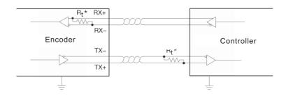
It is a four-wire interface, include the differential lines of TX and RX. And the terminal resistors of the encoder RX lines have been integrated into the encoder. The users only need to configure terminal resistors or choose other impedance matching schemes for TX lines.
