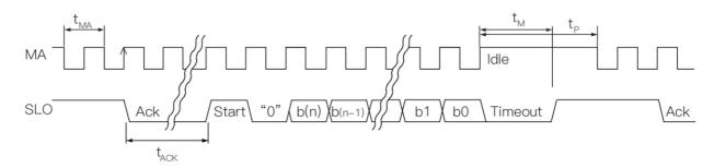
The protocol uses MA as the synchronization clock, and the MA line is high when idle. When the first falling edge of the synchronous clock arrives, the system latches the current data.
