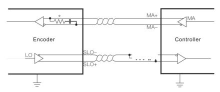
It is a four-wire interface, include the differential lines of MA and SLO. And the terminal resistors of the MA lines have been I ntegrated into the encoder. The users only need to configure terminal resistors or choose other impedance matching schemes for SLO lines.
