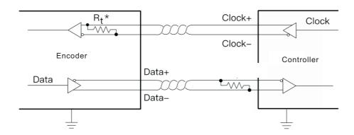
It is a four-wire interface, include the differential lines of Clock and Data. And the terminal resistors of the Clock lines have been integrated into the encoder. The users only need to configure terminal resistors or choose other impedance matching schemes for Data lines.
